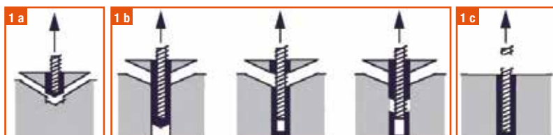
Fig. 1 – Modalità di rottura (da Cook, Kunz, Fuchs e Konz, 1998, "Behavior and Design of Single Adhesive Anchors under Tensile Load in Uncracked Concrete", ACI Structural Journal, V.95, No.1).
